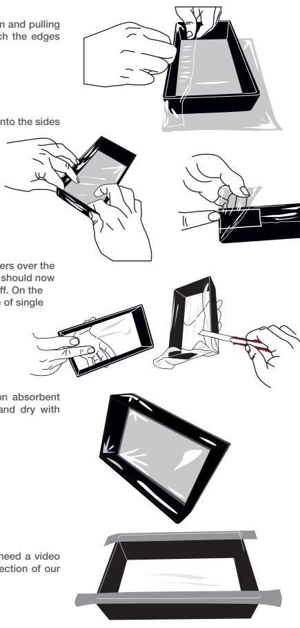
**6.** Apply single sided tape at the corners over the folds to keep the film tight. The vat should now be tensioned. Trim excess edges off. On the short sides of the vat place a piece of single sided tape.
